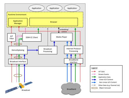
Figure 2: Functional components of a hybrid terminal
